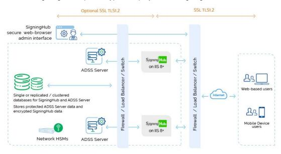
Figure 3 SigningHub Typical Deployment
