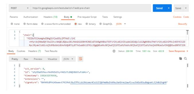
Once it has collected the SCTs, the client application will use this request type (Send SCT) to send the SCTs to Certification Service. The Service issues a certificate embedding the SCTs into it and returns the certificate in response.
